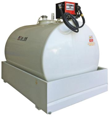
Skid-mounted horizontal cylindrical Diesel tanks manufactured made of carbon steel quality S235JR, watertight electro-welded (submerged arc welding process), provided with anti-roll supports, primed with a rust preventing layer and finished with a layer of white paint. Tanks are delivered pressure-tested and ready-to-use (plug-and-play).
