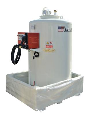
Skid-mounted **vertical cylindrical Diesel tanks** manufactured made of carbon steel quality S235JR, watertight electro-welded (submerged arc welding process), provided with anti-roll sup-ports, primed with a rust preventing layer and finished with a layer of white paint. Tanks are delive-red pressure-tested and ready-to-use (plug-and-play).
