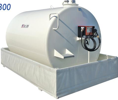
Skid-mounted horizontal cylindrical Diesel tanks manufactured made of carbon steel quality S235JR, watertight electro-welded (submerged arc welding process), provided with anti-roll supports, primed with a rust preventing layer and finished with a layer of white paint. Tanks are delivered pressure-tested and ready-to-use (plug-and-play).
